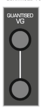
As well an pure analogue Voltage Generator outputs, there is also a Quantised VG output. This will quantise the VG voltage to the nearest semi tone (when using 1V / oct synths).
