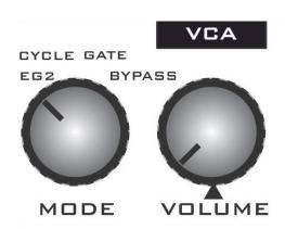
The Voltage Controlled Amplifier (VCA) is the circuit that is used to change the output volume.
