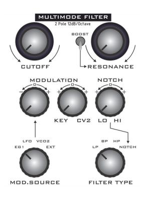
The voltage controlled filter (VCF) is used to alter the tone of the VCOs/Noise and is the heart of what gives an analogue synth its character.
