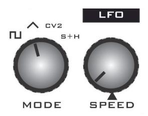
The Low Frequency Oscillator (LFO) is basically identical to a VCO, it is another oscillator, except that it produces periodic wave forms of low frequency, typically subaudio.
