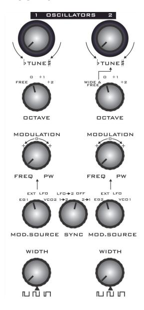
The voltage controlled oscillators (VCOs 1 and 2) produce the raw audio waveform usually used as the initial source for sound creation.
