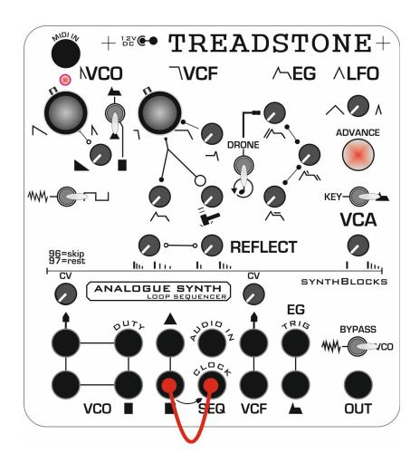
Clocking the Sequencer - using the LFO to clock the internal sequencer.
