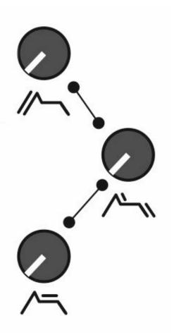
Treadstone features an analogue EG. Although it appears as an ASR type envelope, the 'R' also adjusts 'D' (decay) so you can get pretty good full ADSR style shapes.
