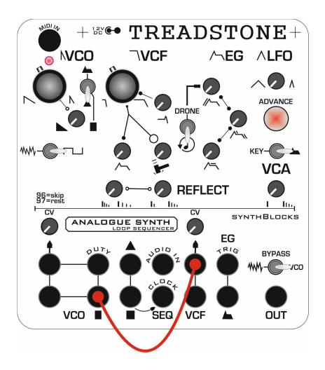
VCF Cross Mod - Use the VCO audio out to modulate the filter cut-off.
