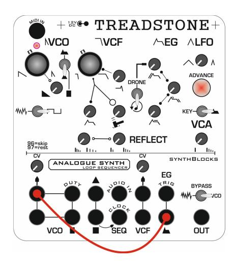
Pitch Sweep - patch EG CV out to Pitch CV in. Adjust the pitch CV mod attenuator to vary the effect. Good for percussive sounds.
