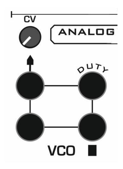
The pitch can be controlled by two external CVs. These are the left two sockets. The top left one also has an attenuator control.
