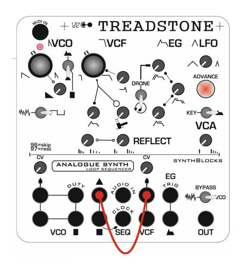
Filter Cut Off Modulation - using the LFO triangle to modulate the filter cut off.
