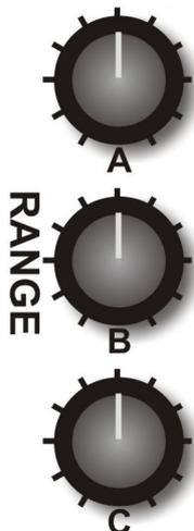
This is used to set the overall level of the CV signal output at the socket. It's an attenuator.
