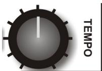
This control sets the speed of the internal clock.
