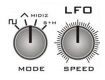
\*Sample and Hold (S+H) is a term that in this instance basically means a modulation is created that has a new random signal level each time the LFO completes a cycle (each time the LFO LED lights up a new modulation level is set)
